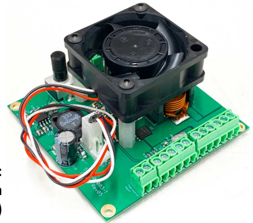
Board size: 70 x 70 x 35mm (including fan)
