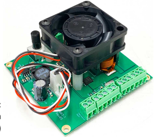
Board size: 70 x 70 x 35mm (including fan)
